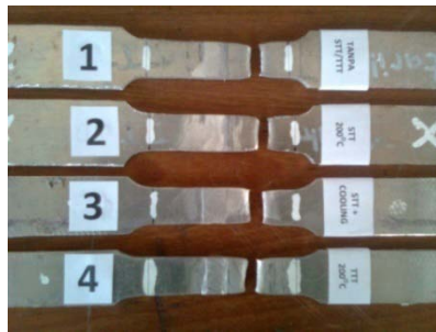
Gambar 11. Hasil uji tarik : (1) tanpa perlakuan, (2) preheat 200°C, (3) STT 200°C, (4) TTT 200°C.
